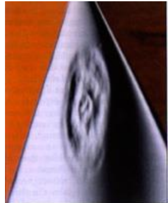
A single laser impact on an aluminium sample.
